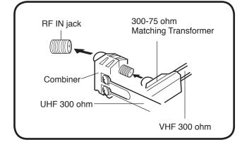
Connect the UHF 300 ohm Twin-lead Wire to the Combiner (not supplied). Connect the VHF 300 ohm Twin-lead Wire to the 300-75 ohm Matching Transformer. Attach the Transformer to the Combiner, then attach the Combiner to the RF IN Jack.
